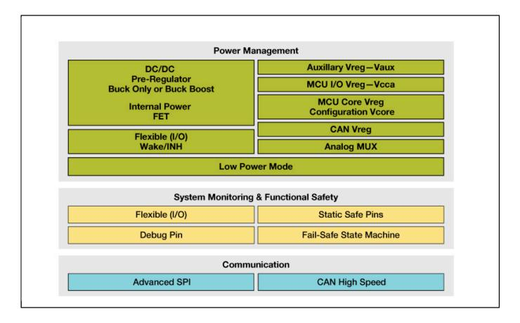
View additional information for Safe SBC with Buck and Boost DC/DC Up to 800 mA on Vcore.
