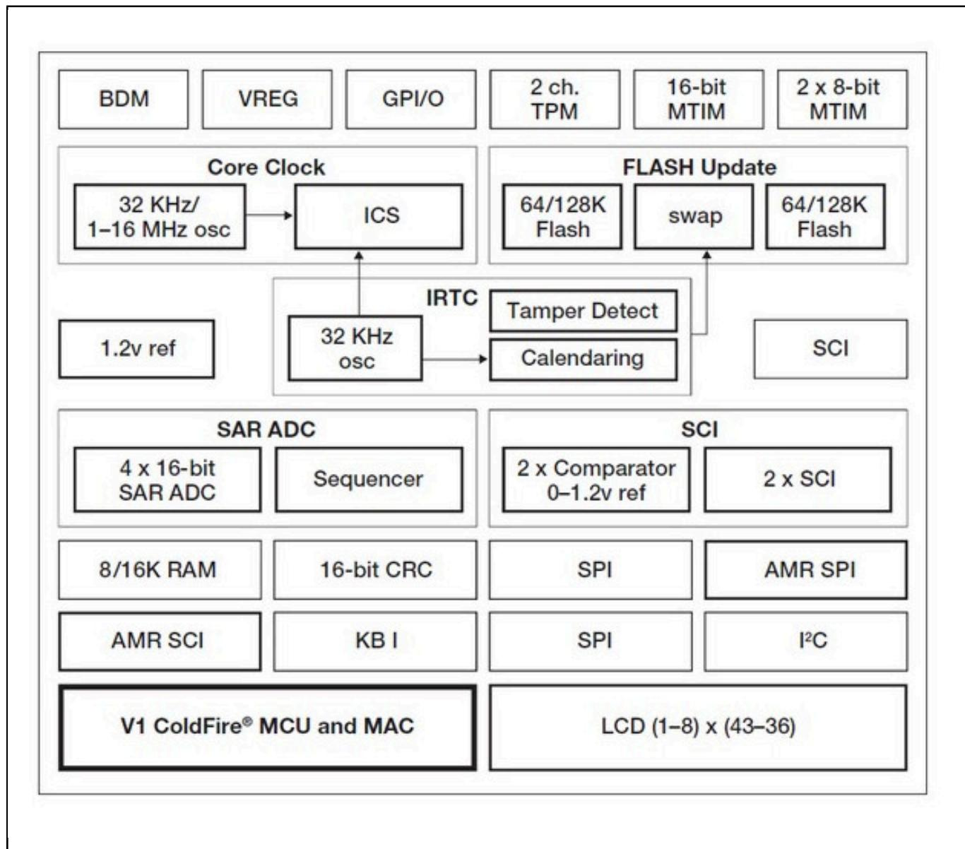
View additional information for [MCF51EM256 32-Bit MCU for Smart Meter Applications](#).
