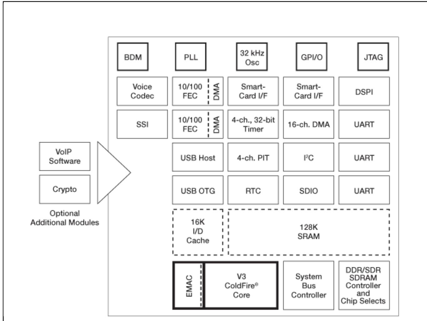
[View additional information for Low-Power MPU with dual Ethernet, USB, and audio sub-system.](#)
