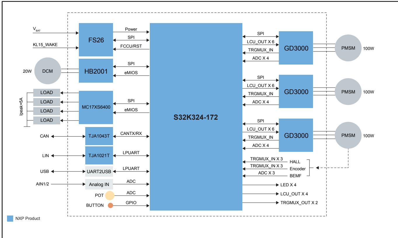
View additional information for [S32K324 Triple Permanent Magnet Synchronous Motor Control \(PMSM\) Reference Design Board](#).
