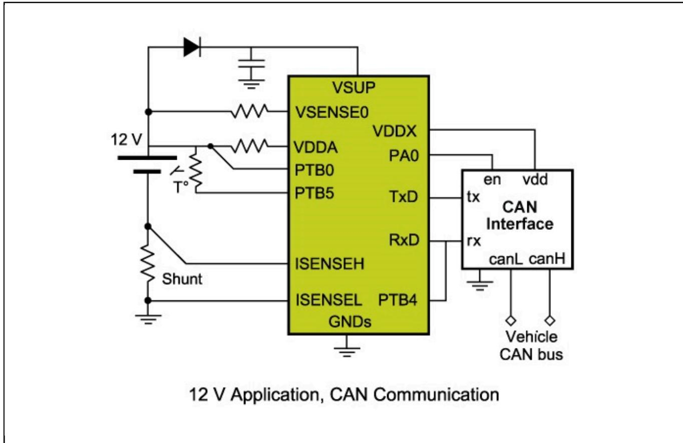
View additional information for [Battery Sensor with CAN and LIN](#).
