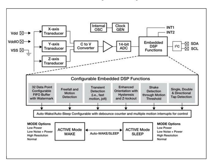
View additional information for ±2g/±4g/±8g, Low g, 14-bit Digital Accelerometer.
