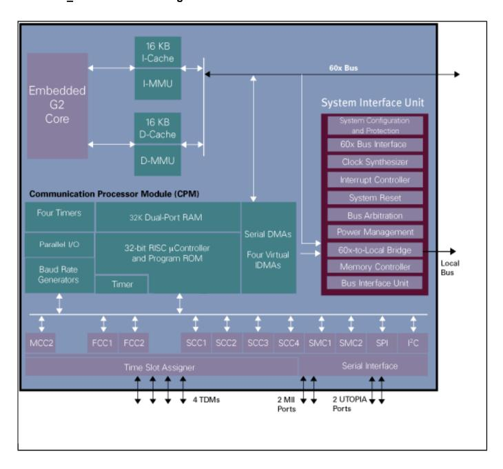
View additional information for PowerQUICC® II Processor with 128-ch. HDLC, UTOPIA II, 10/100 Ethernet.
