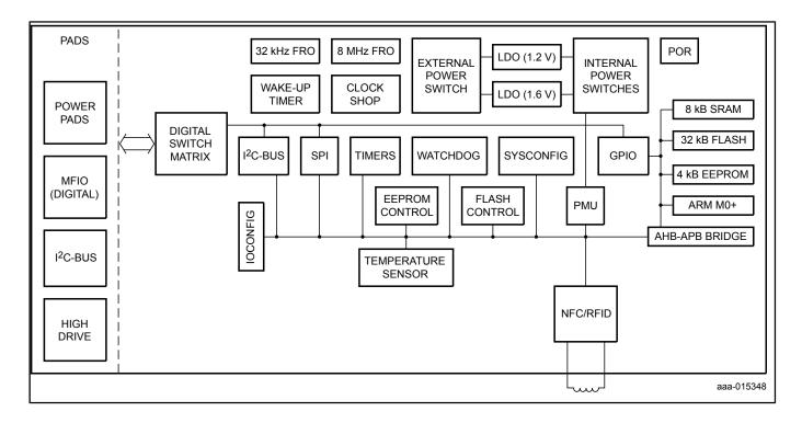
View additional information for NTAG® SmartSensor with Temperature Sensor and Digital IOs.
