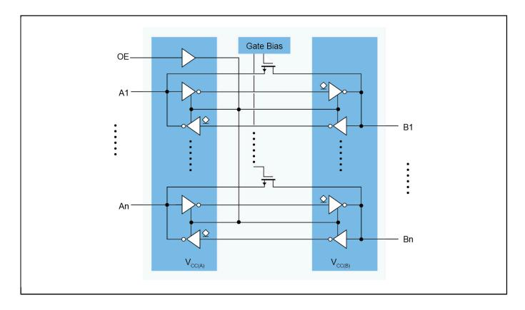
View additional information for 8-Bit Dual-Supply Translating Transceiver (Open-Drain, Auto-Direction Sensing).
