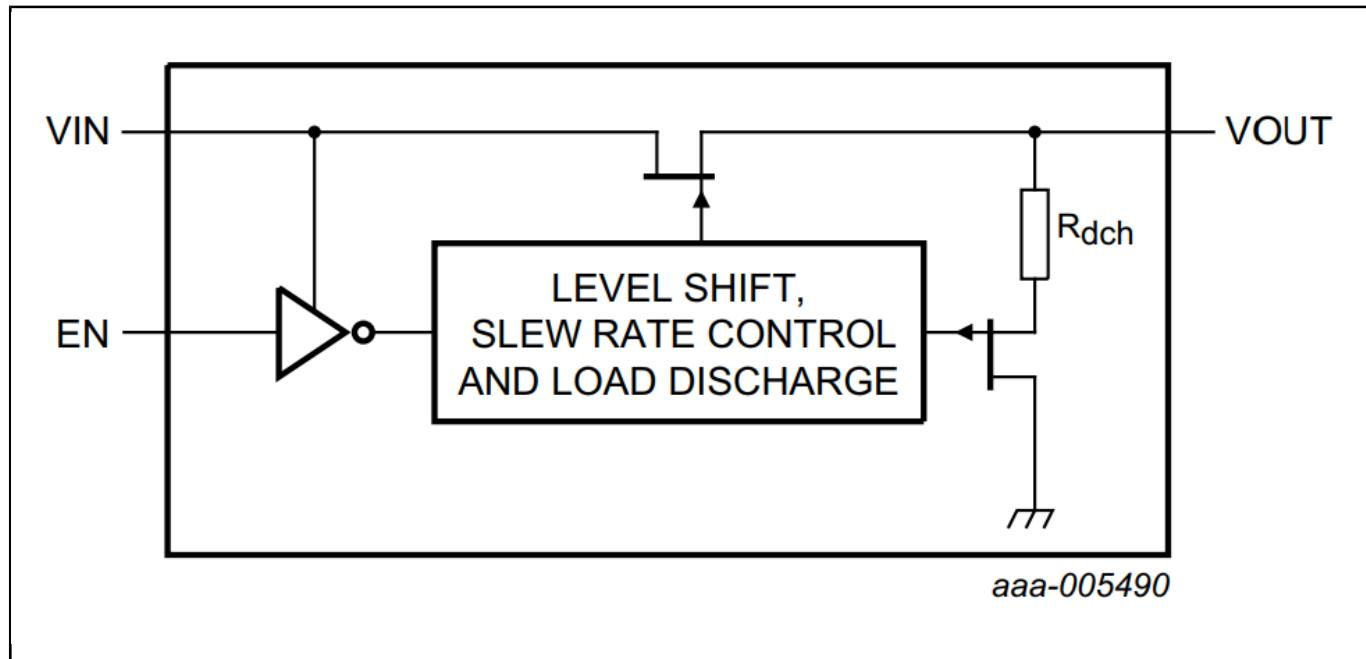
View additional information for [Logic-Controlled High-Side Power Switch](#).
