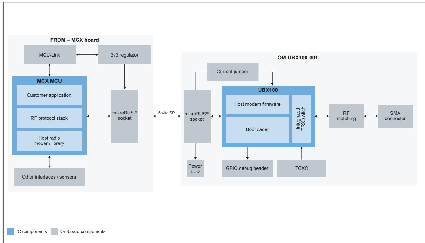
View additional information for [Breakout Board for UBX100 Sub-GHz RF Transceiver](#).
