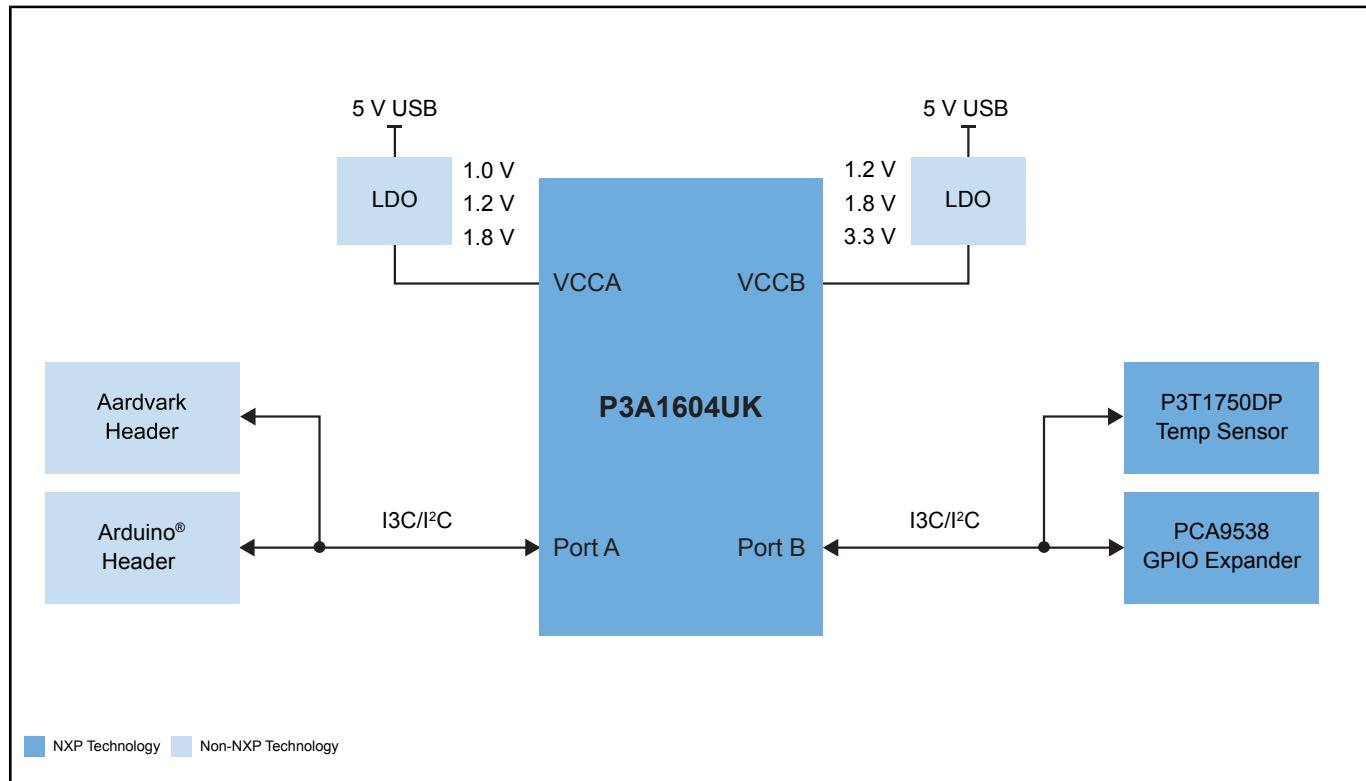
[View additional information for 4-Bit Voltage Level Translator Arduino® Shield Evaluation Board.](#)
