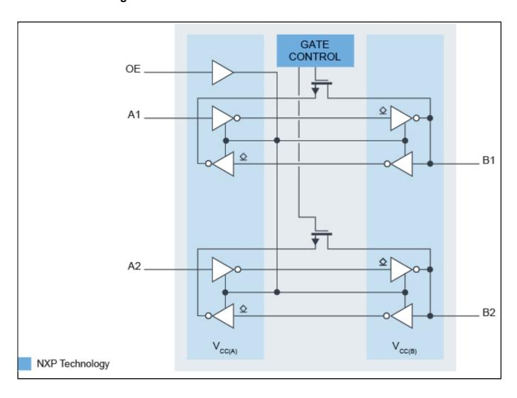
View additional information for 2-Bit Dual Supply Bidirectional I3C/I2C-Bus and SPI Voltage-Level Translator.
