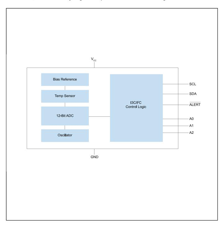
View additional information for I3C/I2C-Bus, ±1 °C Accuracy, Digital Temperature Sensor.
