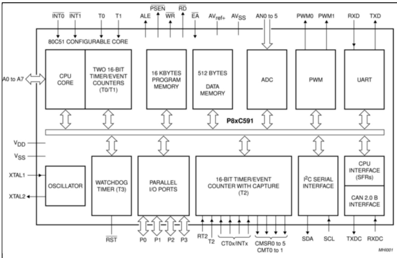
[View additional information for Single-Chip 8-Bit Microcontroller with CAN Controller.](#)
