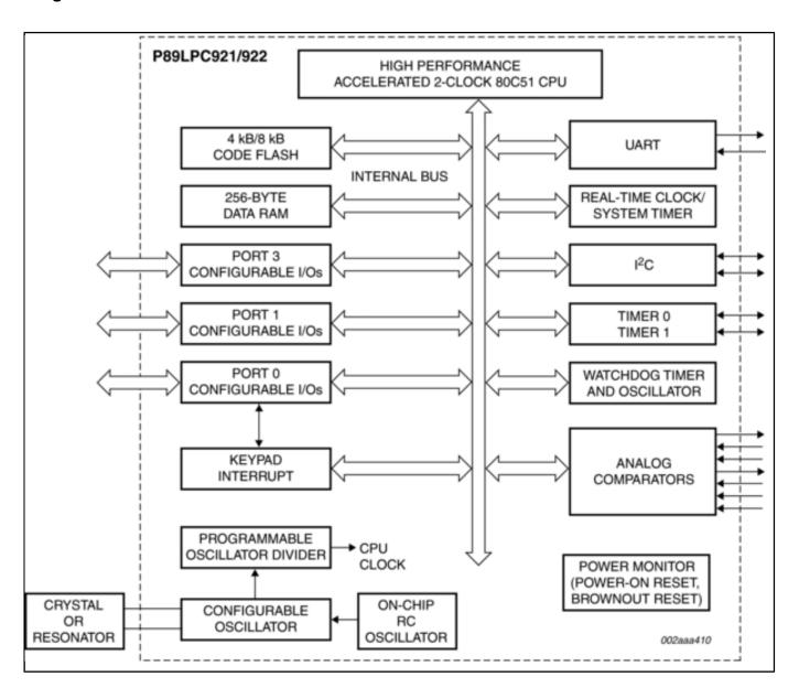
View additional information for 8-Bit Microcontrollers with Accelerated Two Clock 80C51 Core 2 KB 3 V Flash with 8-Bit A/D Converter.
