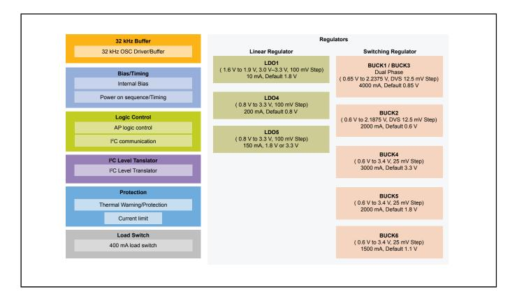
View additional information for PCA9451A Power Management IC for i.MX 93x/91x Application Processor.
