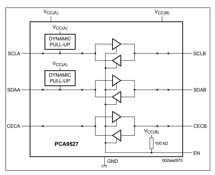
View additional information for Three-Channel Bidirectional Bus Extender for HDMI, I2C-Bus and SMBus.
