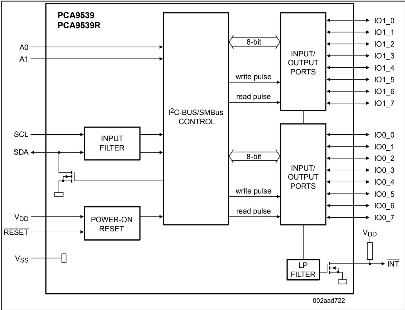
**PCA9539BS, PCA9539D, PCA9539PW, PCA9539RBS, PCA9539RPW Block Diagram**
