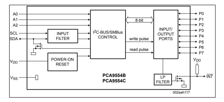
View additional information for Low-Voltage 8-Bit I<sup>2</sup>C-Bus and SMBus Low Power I/O Port with Interrupt, Weak Pull-Up.
