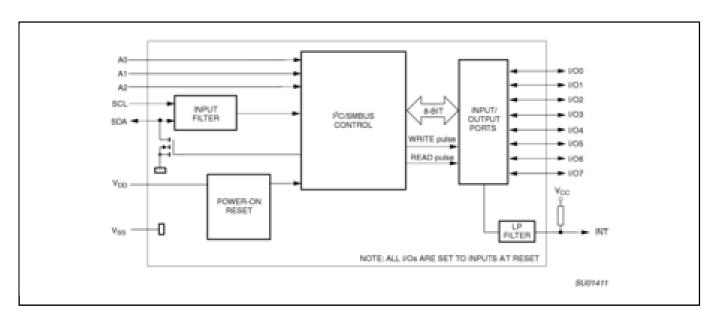
View additional information for 8-Bit I<sup>2</sup>C-Bus and SMBus I/O Port with Interrupt.
