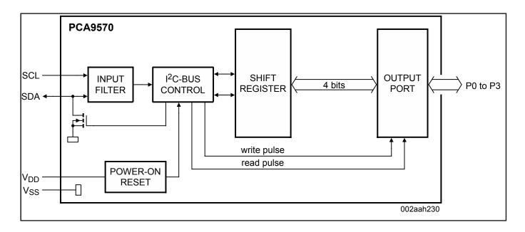
View additional information for Remote 4-Bit General Purpose Outputs for 1 MHz I<sup>2</sup>C-Bus.
