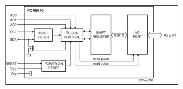
View additional information for Remote 8-Bit I/O Expander for Fm+ I<sup>2</sup>C-Bus with Reset.
