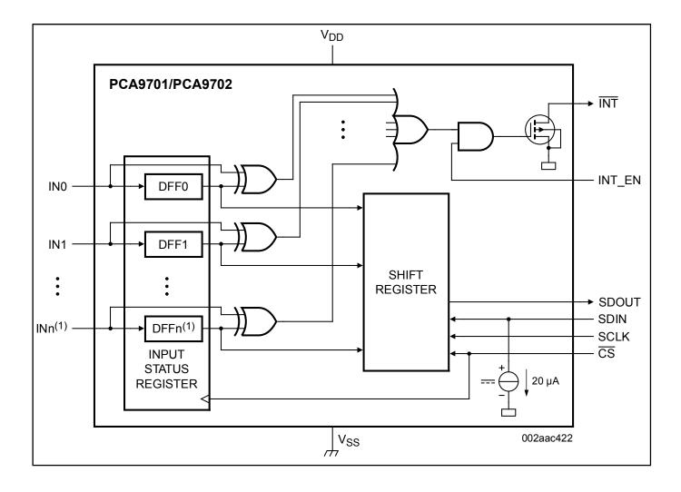
View additional information for 18 V Tolerant SPI 16-Bit/8-Bit GPI with INT.
