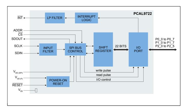
View additional information for 22-Bit SPI I/O Expander with Agile I/O Features.
