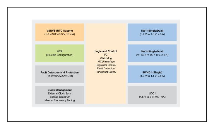
View additional information for Multi-Channel (5) PMIC for Automotive Applications – 4 High Power and 1 Low Power, Fit for ASIL B Safety Level.
