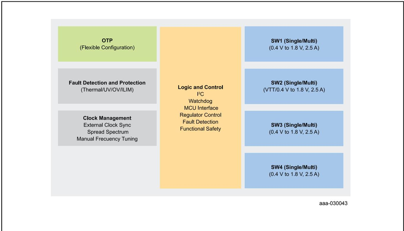
View additional information for [Multi-Channel \(4\) PMIC for Automotive Applications – 4 High Power, Fit for ASIL B Safety Level](#).
