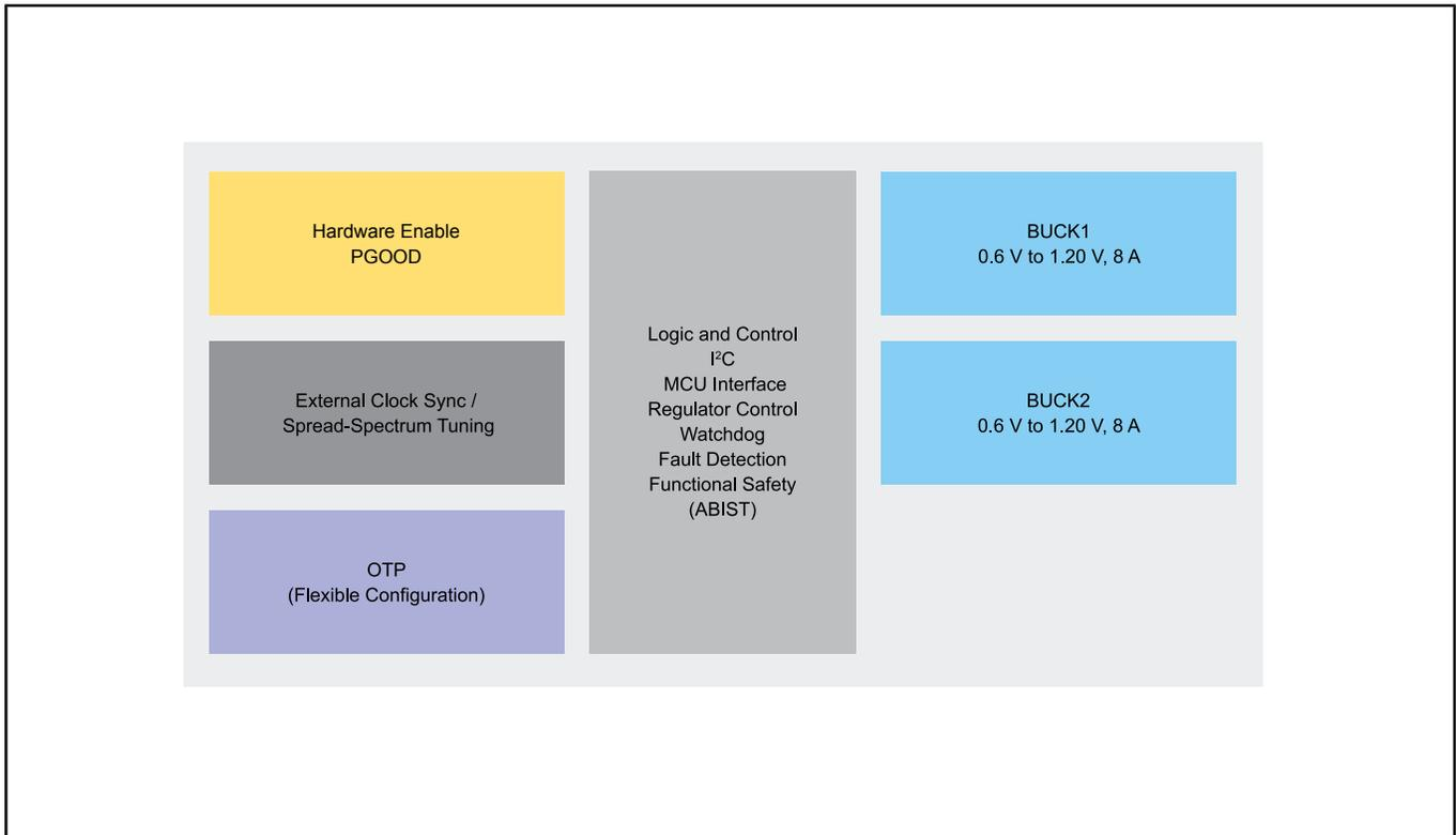
View additional information for [Dual-Channel PMIC for Automotive Applications – 2 High Efficient LVBUCK, Fit for ASIL B Safety Level](#).
