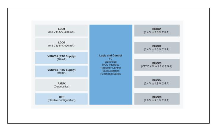
View additional information for 7-Channel Power Management Integrated Circuit for High Performance Applications, Fit for ASIL B Safety Level.
