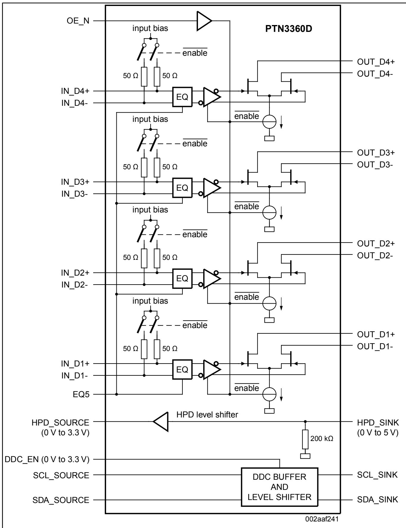
[View additional information for Enhanced Performance HDMI/DVI Level Shifter with Active DDC Buffer, Supporting 3 Gbit/s Operation.](#)
