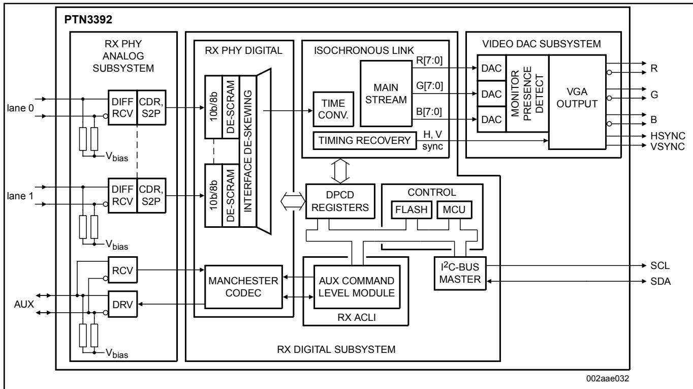
[View additional information for Two-Lane Displayport to VGA Adapter IC.](#)
