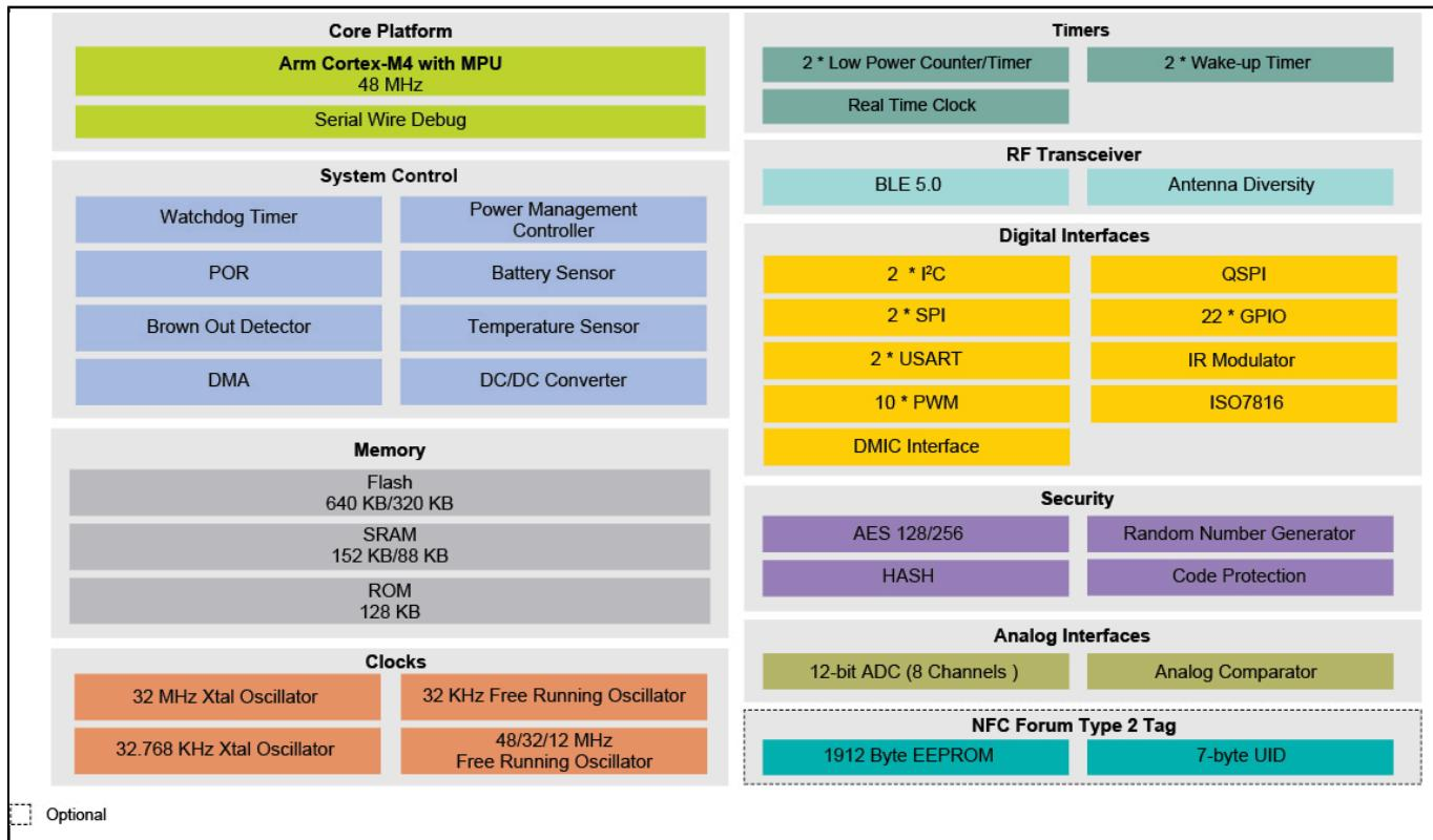
View additional information for [QN9090/30: Bluetooth Low-Energy MCU with Arm®Cortex®-M4 CPU, Energy Efficiency, Analog and Digital Peripherals and NFC Tag Option](#).
