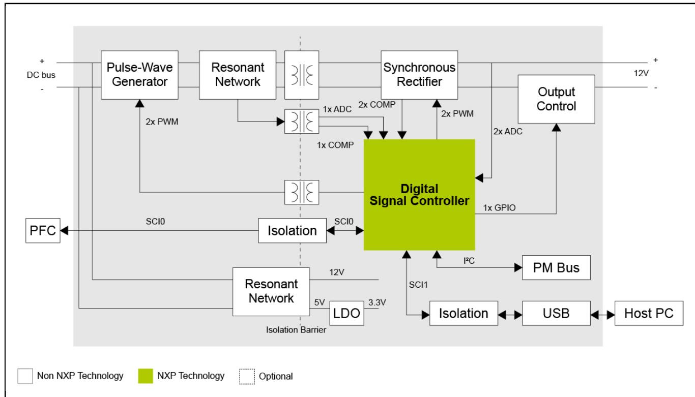
View additional information for [LLC Resonant Converter with Sync Rectifier](#).
