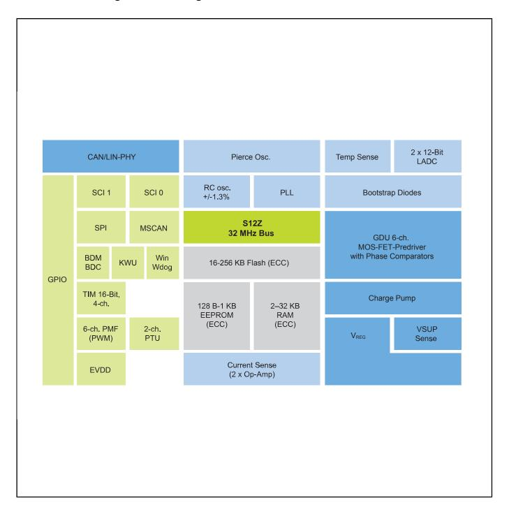
View additional information for S12ZVM Mixed-Signal MCU for Automotive and Industrial Motor Control Applications.
