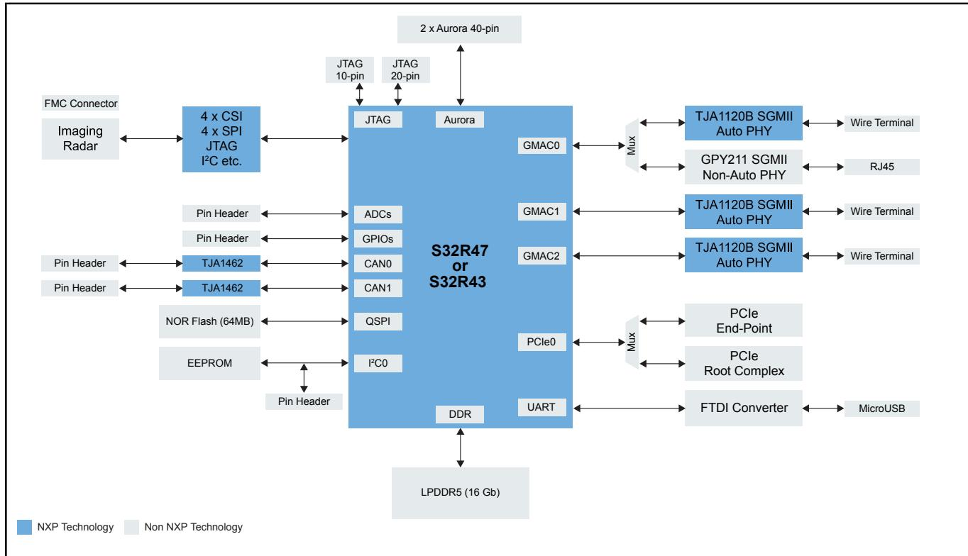
[View additional information for S32R47 Imaging Radar Processor Evaluation Board.](#)
