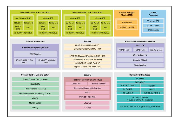
S32Z and S32E Real-Time Processors Software Block Diagram
