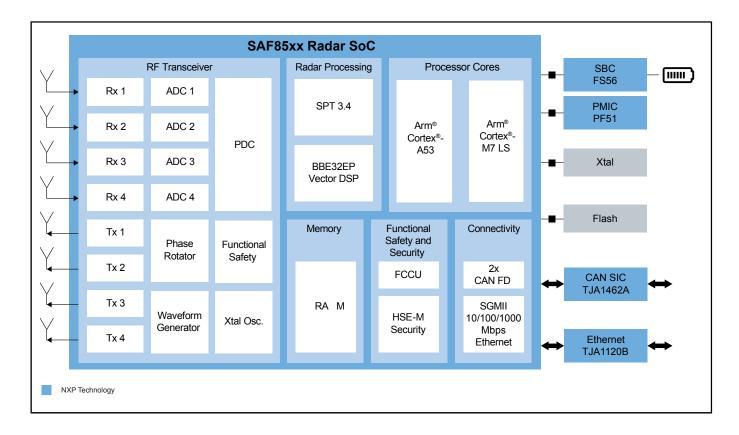
View additional information for High Performance 77GHz RFCMOS Automotive Radar One-Chip SoC.
