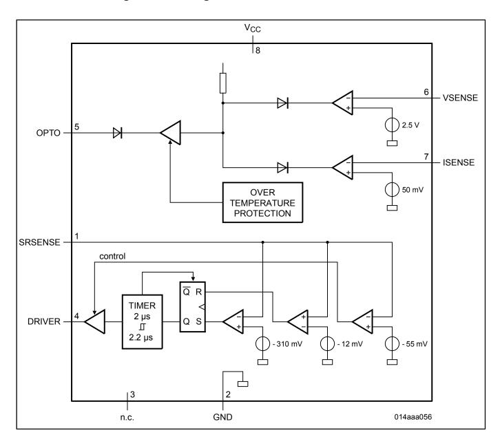
View additional information for Synchronous Rectification Controller with Integrated Feedback and Protection.
