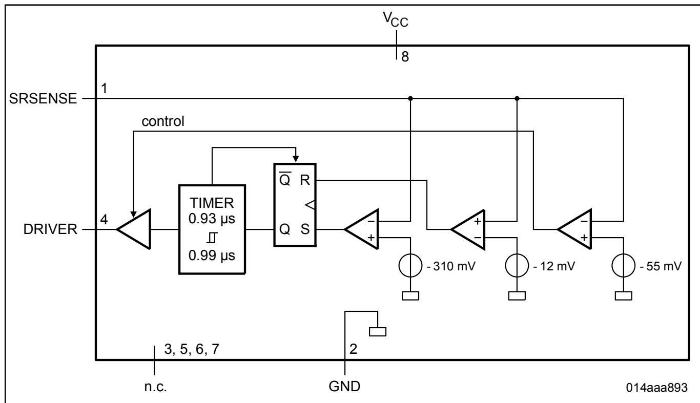
[View additional information for Synchronous Rectification Controller Suitable for Both High-Side and Low-Side Control.](#)
