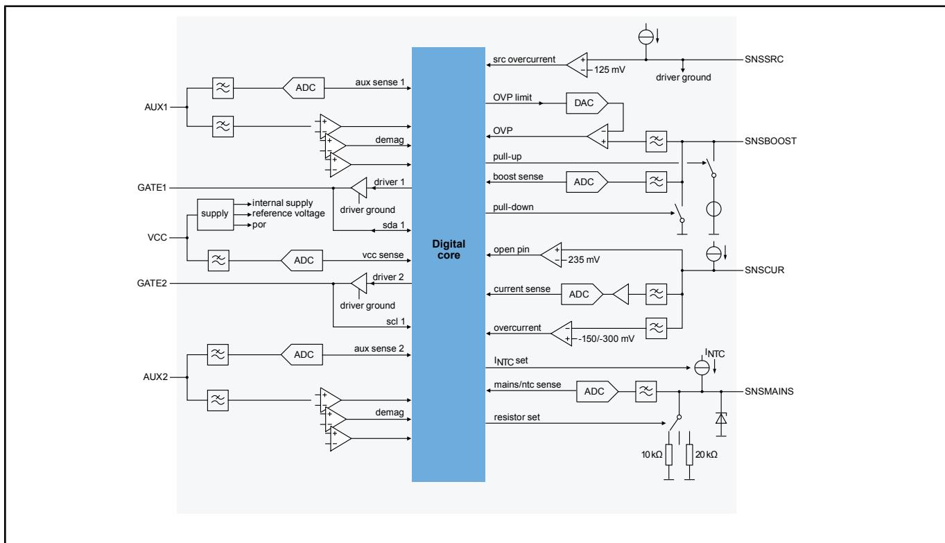
[View additional information for TEA2376xT, Digital Configurable Interleaved PFC Controllers.](#)
