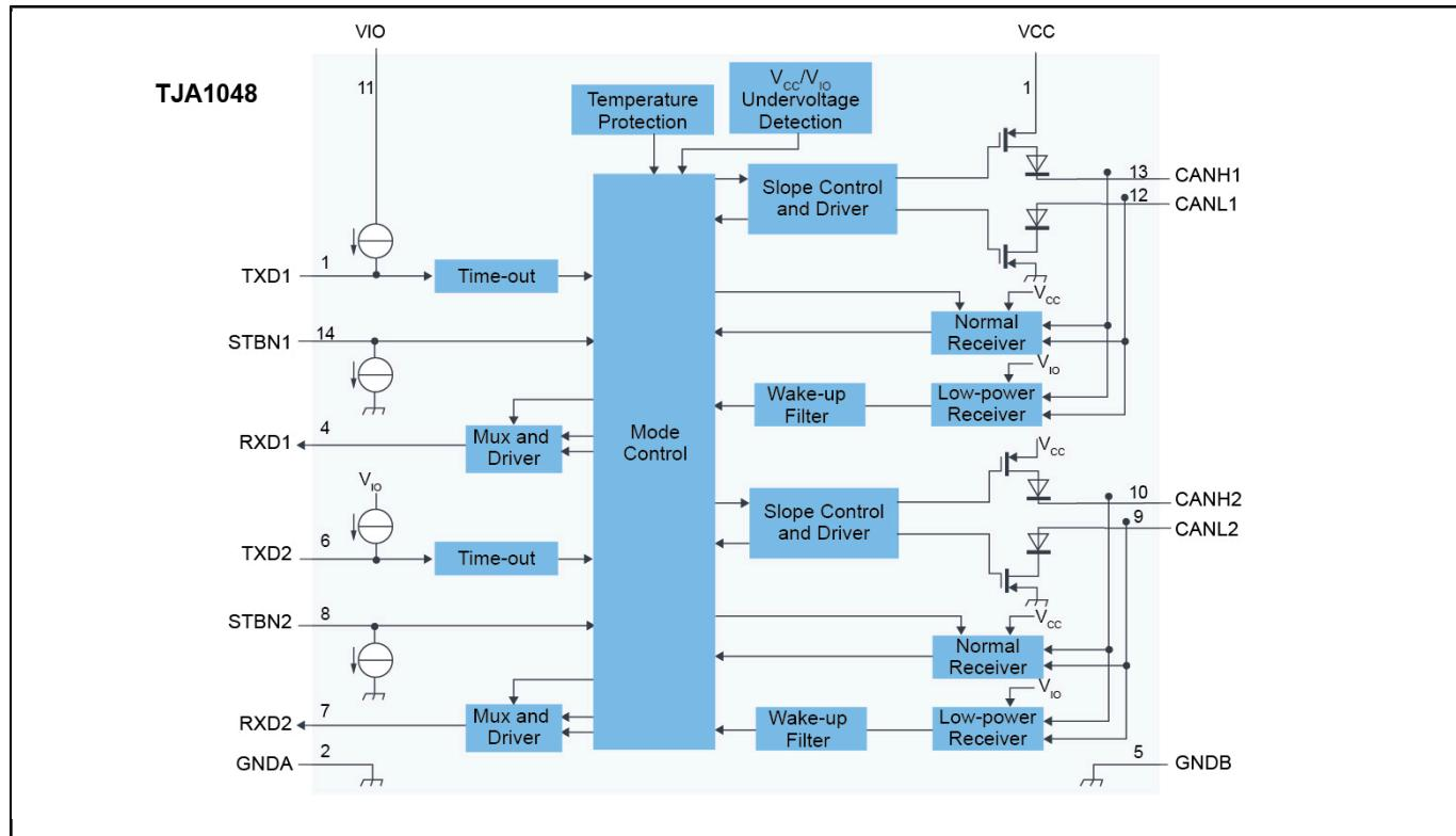
[View additional information for Dual High-Speed CAN Transceiver with Standby Mode.](#)
