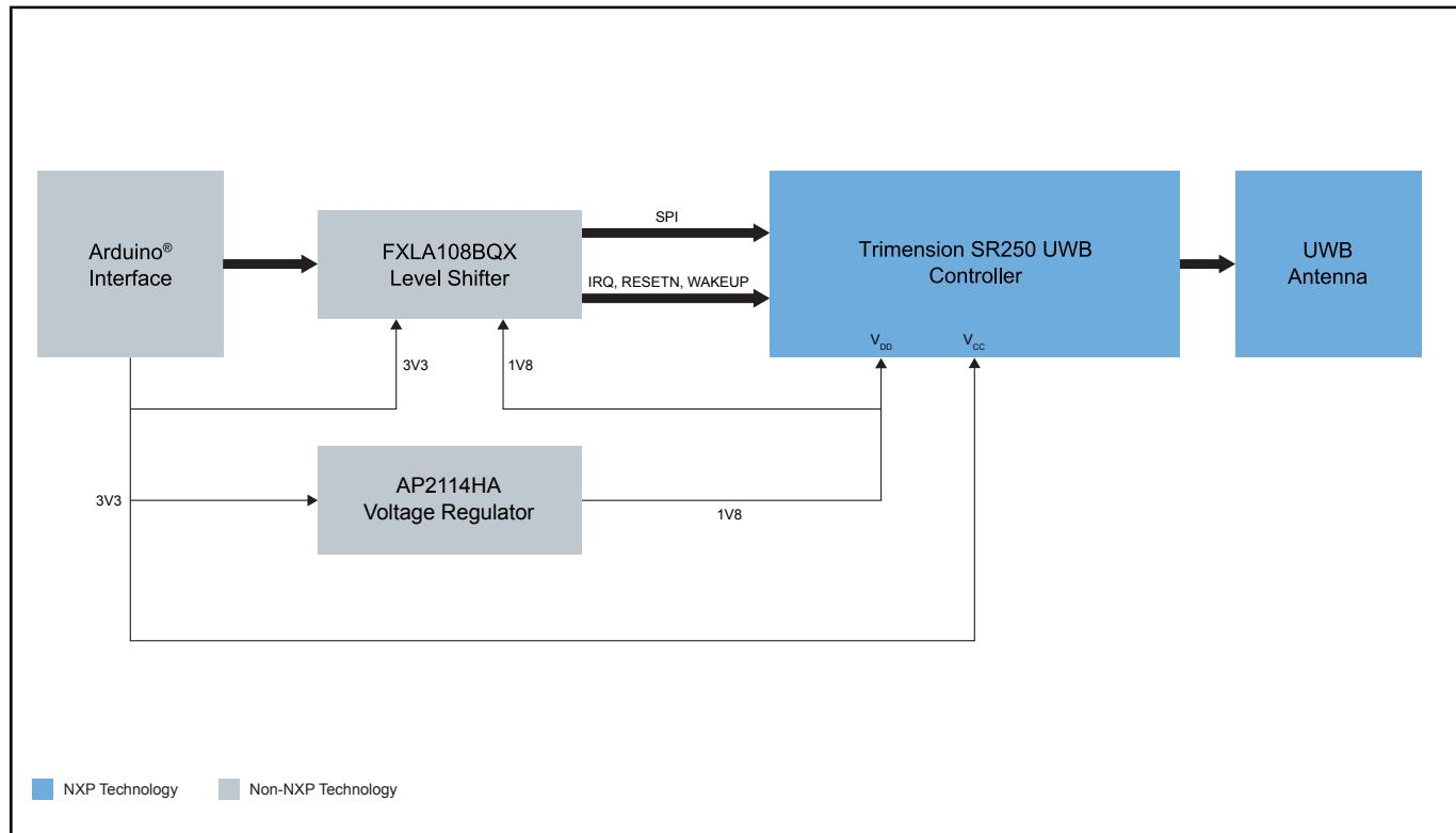
[View additional information for Trimension SR250 Development Board for UWB Ranging and Radar Applications.](#)
