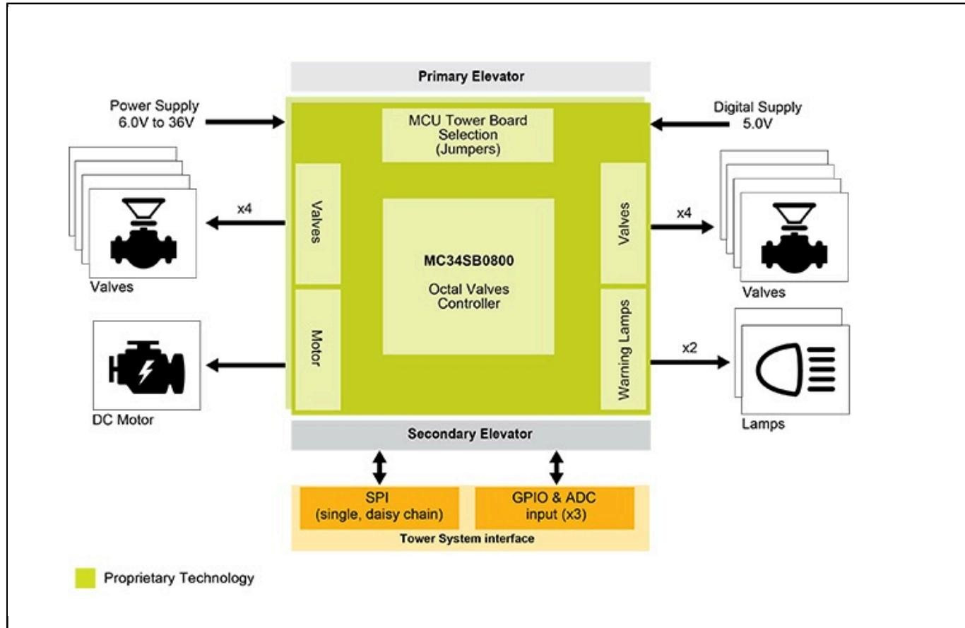
[View additional information for Tower Board - SB0800, Octal Valve/Pump Controller SoC.](#)
