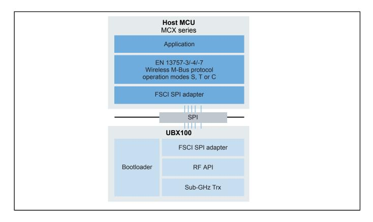
View additional information for UBX100 Sub-GHz Wireless M-Bus Solution.
