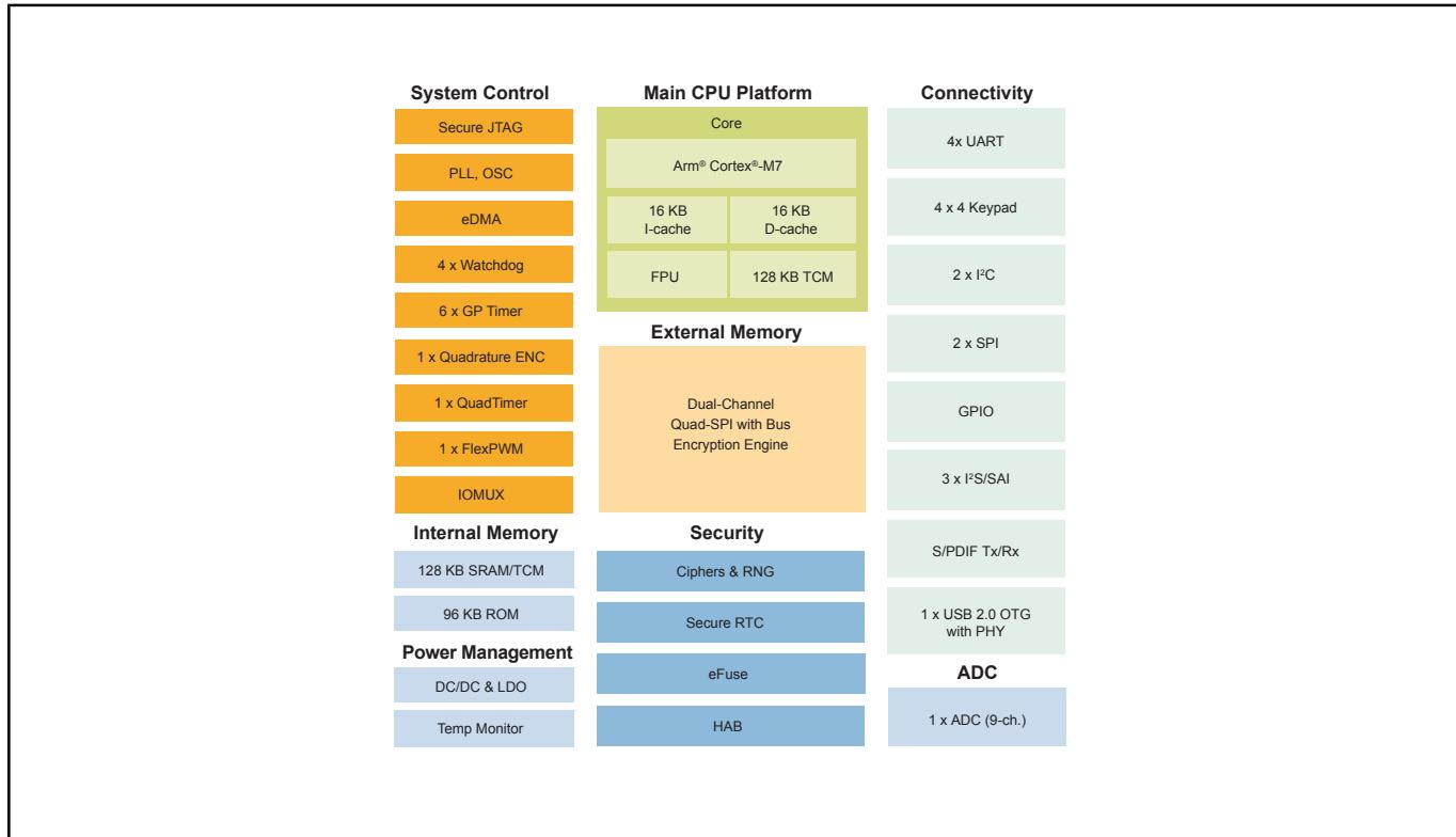
View additional information for [i.MX RT1015 Crossover MCU with Arm® Cortex®-M7 Core Operating Up to 500 MHz](#).
