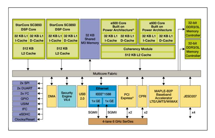
View additional information for QorlQ® Qonverge BSC9132 Dual-Core Processor and Dual-Core DSP.
