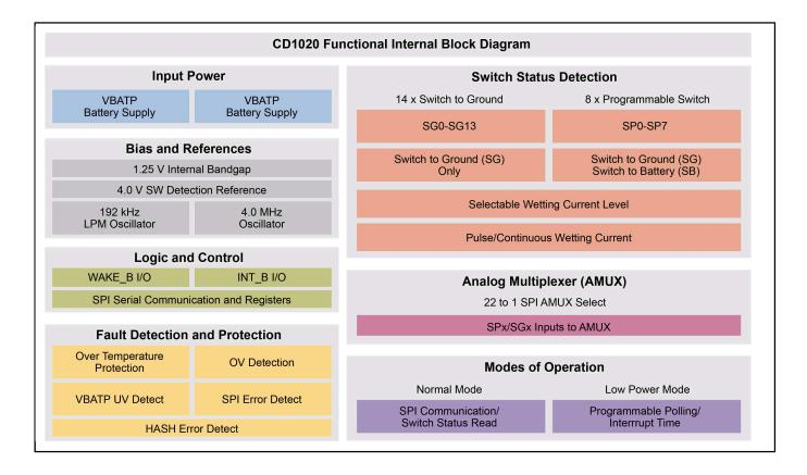
View additional information for Low-Cost 22-CH Multiple Switch Detect Interface.
