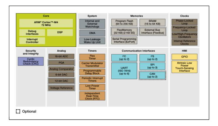
View additional information for Kinetis® K10-72 MHz, Mixed-Signal Integration Microcontrollers (MCUs) based on Arm® Cortex®-M4 Core.
