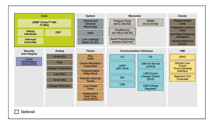
View additional information for Kinetis® K40-72 MHz, Mixed-Signal Integration Microcontrollers based on Arm® Cortex®-M4 Core.
