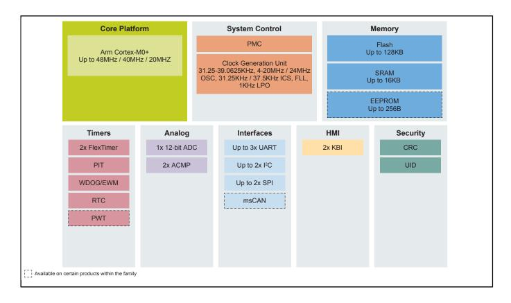
View additional information for Kinetis® KE02-40 MHz, Entry-Level Microcontrollers (MCUs) based on Arm® Cortex® -M0+ Core
